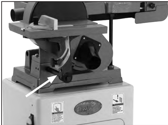
Figure 86. Table support rod lubrication.
